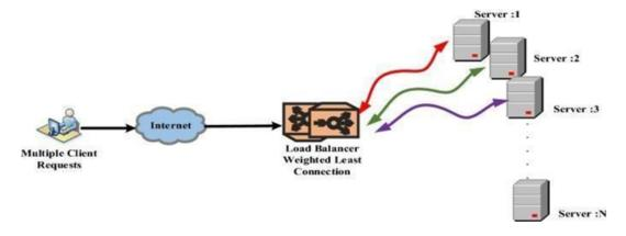
Figure 3.3: Weighted Least Connections in Load Balancing
