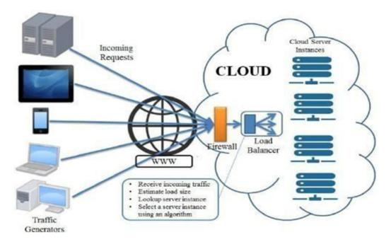
Figure 3.1: Load Balancing in Cloud
