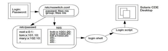
Figure 5.4: Solaris User Login Process
