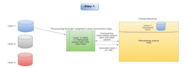
Figure 3.5: Working mechanism of algorithm with User 1 requesting
