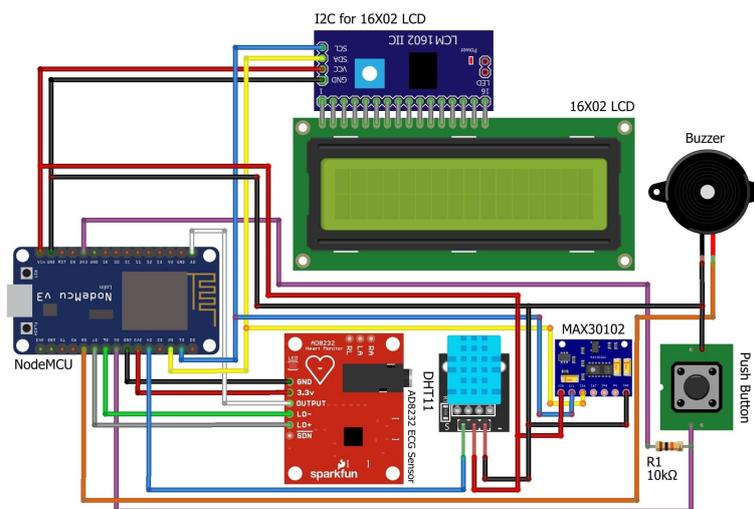
Figure 4.7: Circuit Diagram of Health Monitoring IoT Device
