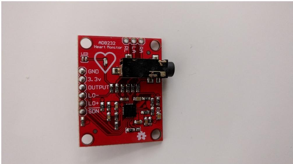
Figure 4.3: AD8232 Heart Rate Sensor
