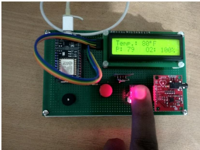
Figure 4.8: Pulse rate and blood oxygen checking
