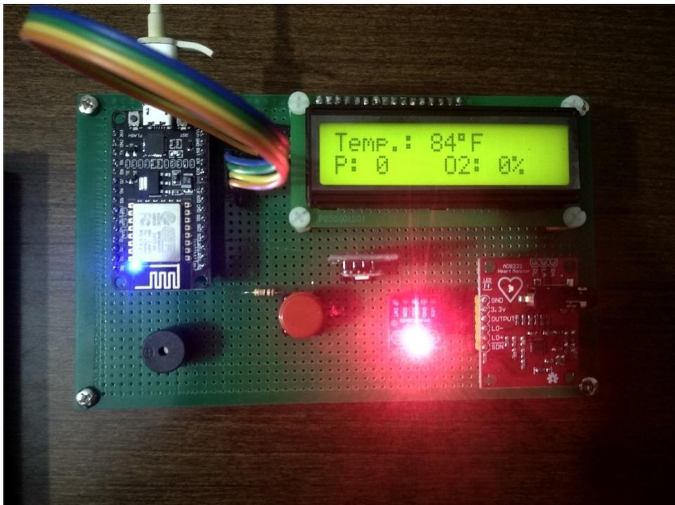
Figure 4.1: Health Monitoring IoT Device
