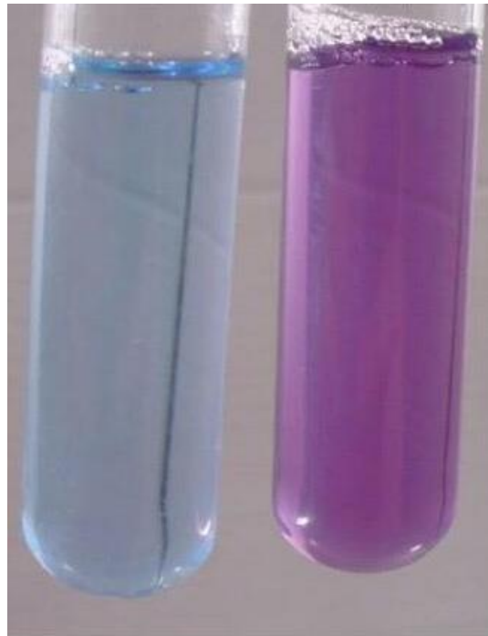
Figure 23: Protein Concentration by Biuret's Assay: Left: Blank; Right: Positive result
