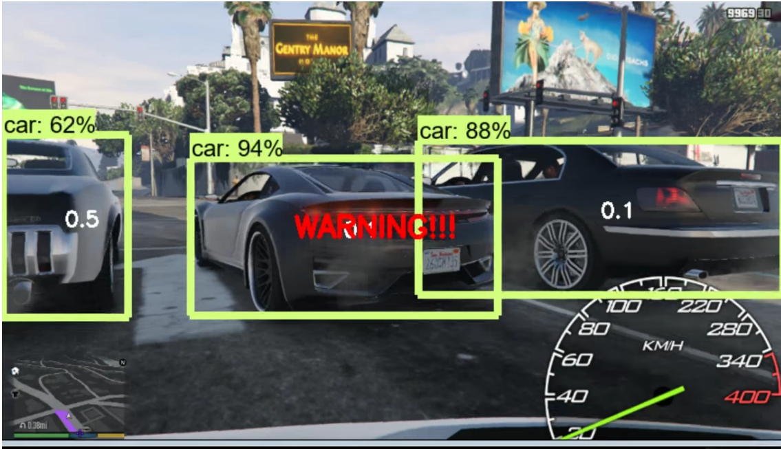
Figure 4.11: Braking Situation in terms of Distance Calculation in GTA V Environment [52]
