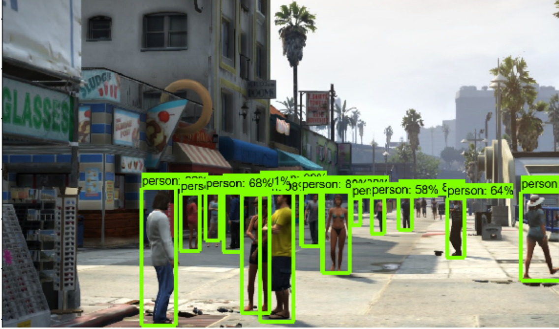
Figure 4.3: Image Classification through Faster R-CNN: Pedestrian [52]
