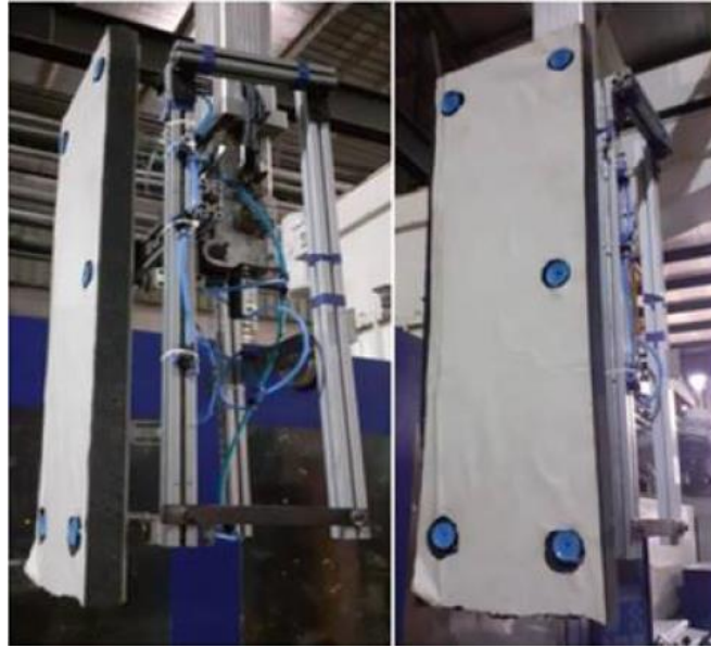
Figure-4.2(c): Normal robot converted to IML robot
