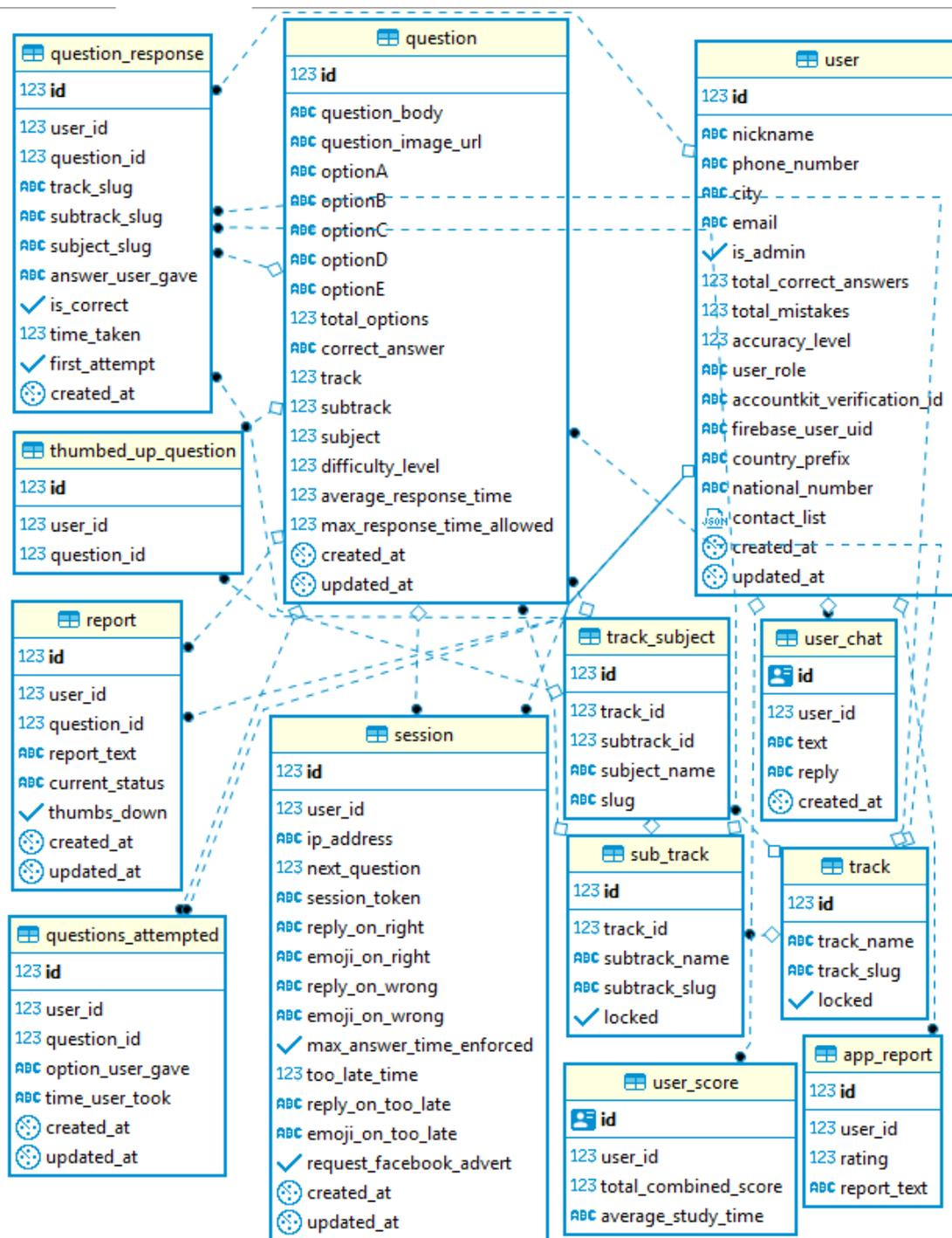
**Figure 3.7:** ER Diagram of the Database used on the Application Level for Data Analysis and Interpretation Modules
