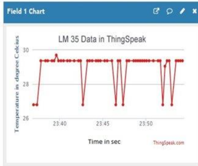
Figure 5.10.1: Temperature Control Monitoring using LM35 Sensor
