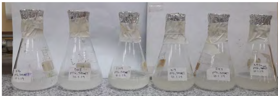
Figure 17 Growth of isolates in MS 2 broth (pH 6 with 250 ul Tween 20) with 0.1% LDPE
