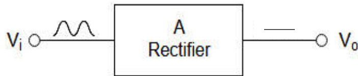
Fig. 6.4 General Block Diagram of a Rectifier
