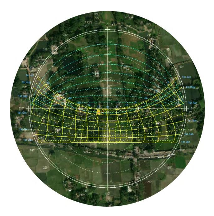
Figure 3.2.2.1: showing site and solar orientation and stereographic diagram of it. Digital Globe, 2018
