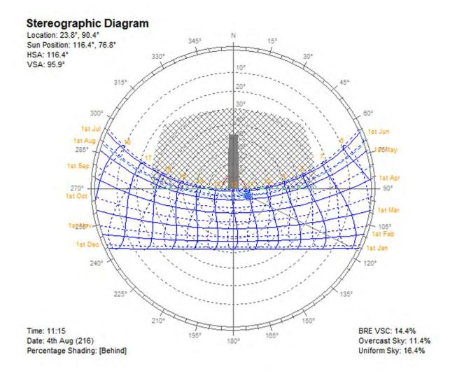
Figure: 3.1.3.4 showing stereographic Diagram of solar positioning and shadow cast using ECOTECT ANALYSIS, Nurul. August 4, 2018.
