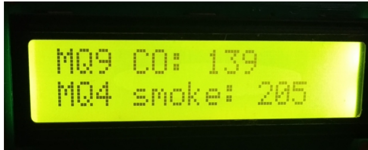
Fig. 5.1 Output value of MQ-4 and MQ-9 gas sensor in LCD display
