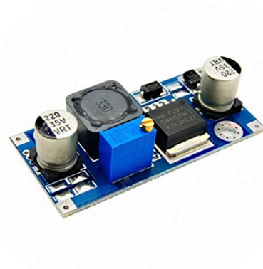
Fig. 4.12 DC-DC Buck Converter
