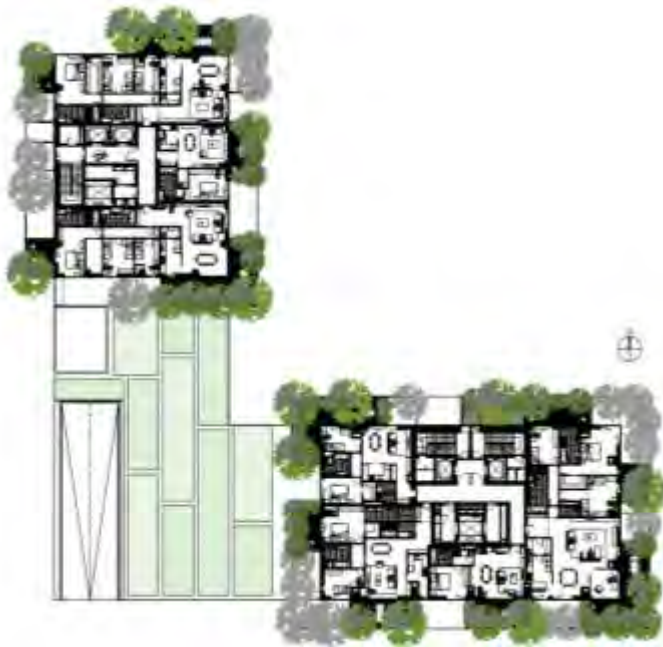
Figure 4.2.5: Typical plan showing the terrace with cantilevered from the main tower plans
