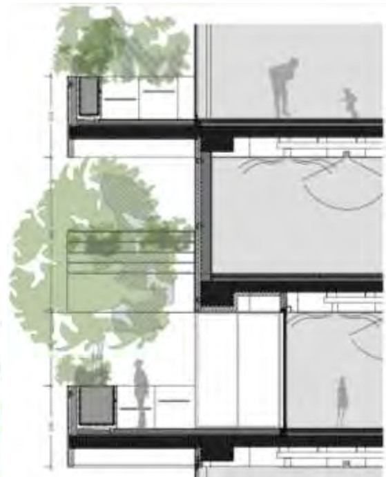
Figure 4.2.6: Detailed section showing cantilevered terrace
