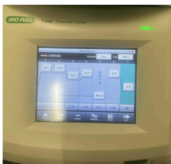
Figure 1: Thermal cycler program used for colony PCR amplification. The protocol included an initial denaturation at 95 °C for 10 min to lyse bacterial cells, followed by 30 cycles of denaturation at 95 °C for 30 s, annealing at 58 °C for 30 s, and extension at 72 °C for 1 min, with a final extension at 72 °C for 7 min. The conditions enabled direct amplification of target DNA from bacterial colonies. (Picture taken from Brac University Molecular Lab.)
