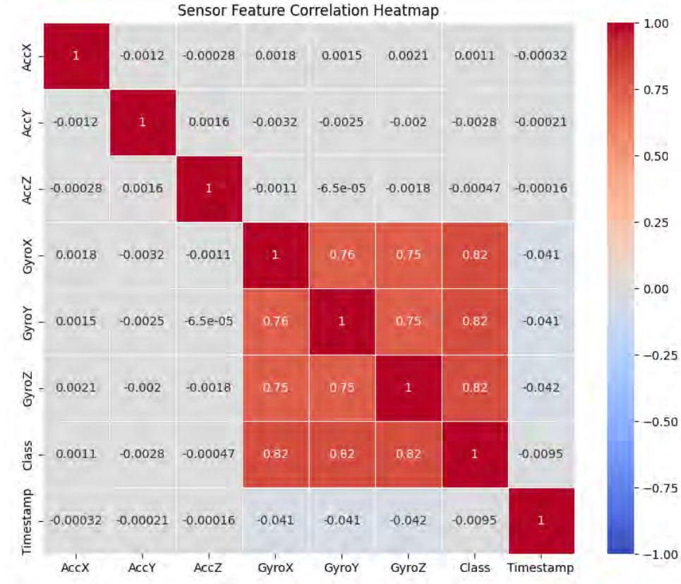
Figure 4.4: Sensor Feature Correlation Heatmap (Accelerometer and Gyroscope Data) – Shows the high degree of interdependency among motion sensors, which justifies the use of a unified sensor-based neural network for behavioral detection.
