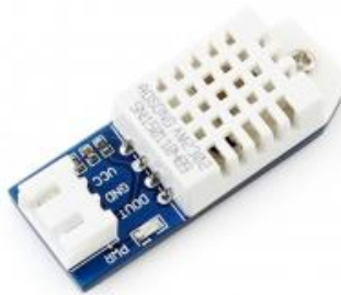
Figure 2.12 Moisture and temperature sensor (DHT22) (Source: Wikipedia).
