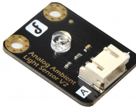
Figure 2.10 Analog ambient light sensor(Source: Wikipedia).
