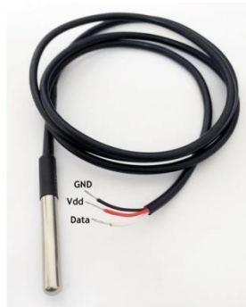
Figure 2.13 Soil temperature sensor DS18B20(Source: Wikipedia).
