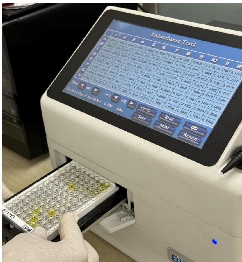
Figure 28: Measurement of Absorbance using Microplate Reader
