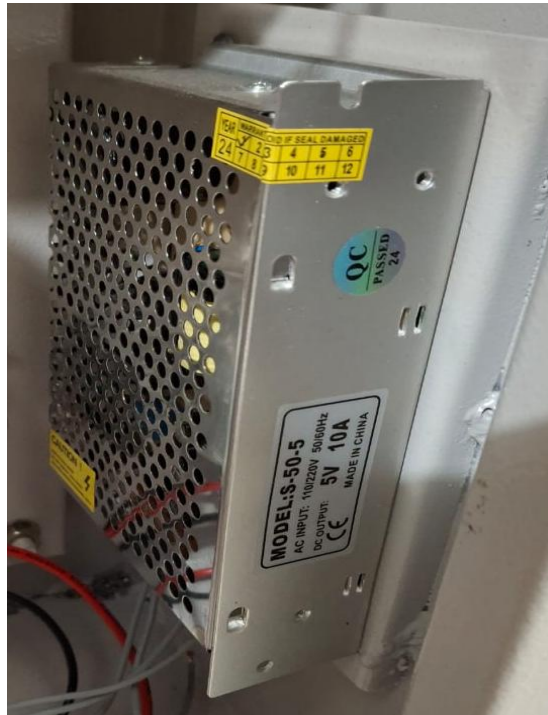
Figure 5.4: Power Supply 220VAC- 5VDC
