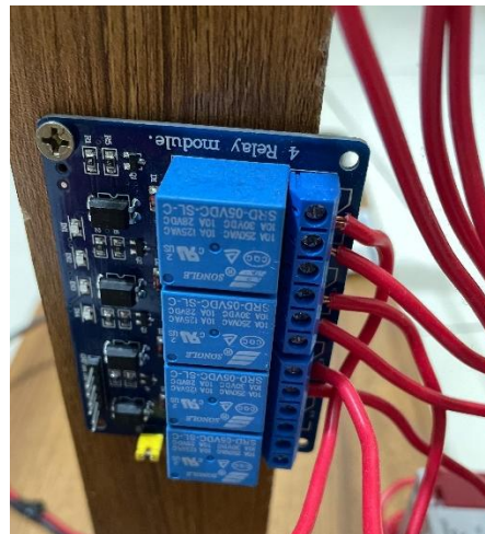
Figure 5.27: 4 channel Relay that turn on/off the 3-phase power supply.
