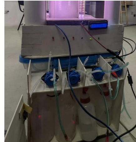
Fig.35: Peristaltic Pump Integration to Supply Nutrient
