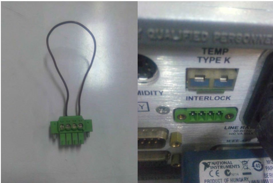
Fig 2.15: Interlock connector with pins 1 and 3 shorted (left) and the back panel showing interlock section (right)
