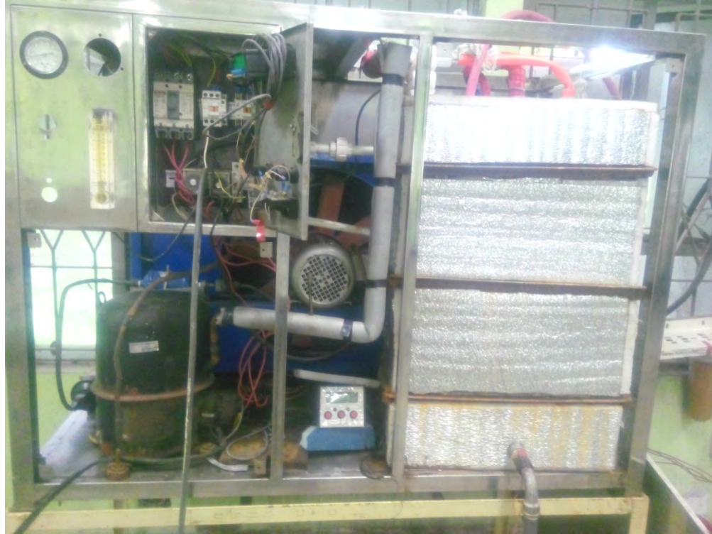
Fig 2.8: The mini-coater cooling system after necessary modifications
