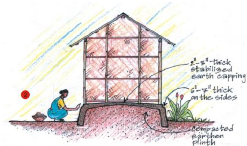
Figure 39. Cement-stabilized earthen plinth (Source: adpc report, 2005)
