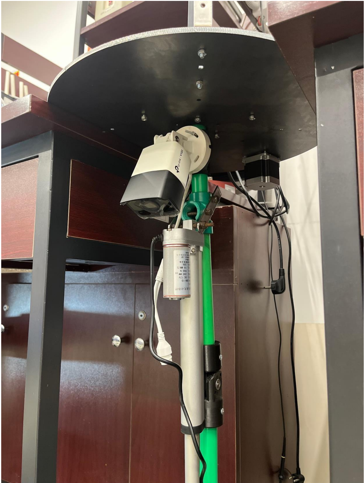
Figure 5.4 Working Prototype (IP Cam and Base Rotation Mechanism)
