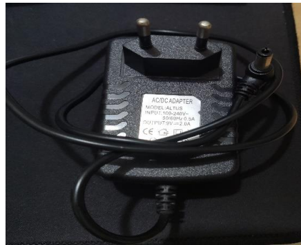
Fig 2.10: An Illustration of Power Adapter
