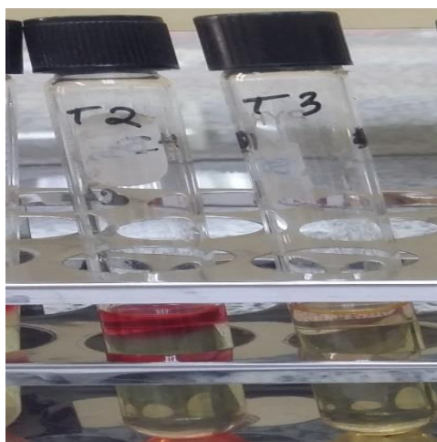
Figure 3.3.3: The sample T2 at the left showing the positive result and the sample T3 on the right shows the negative result for Voges-Proskauer test .
