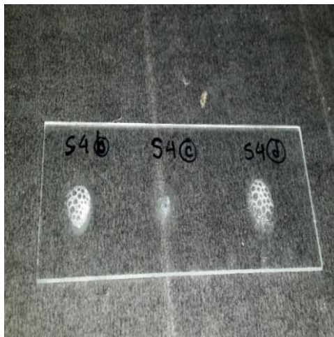
Figure 3.3.6: The sample S4 (b) and S4 (d) shows positive result bur sample S4 (d) shows false negative result for Catalase test .
