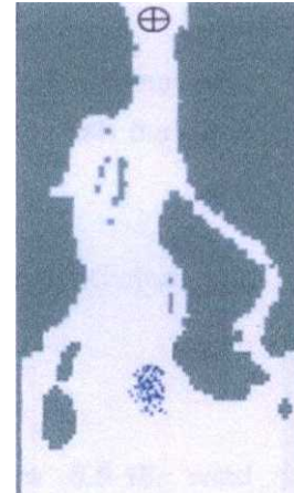
Figure: Variation of oil position with change in wind coefficients after 12 hours
