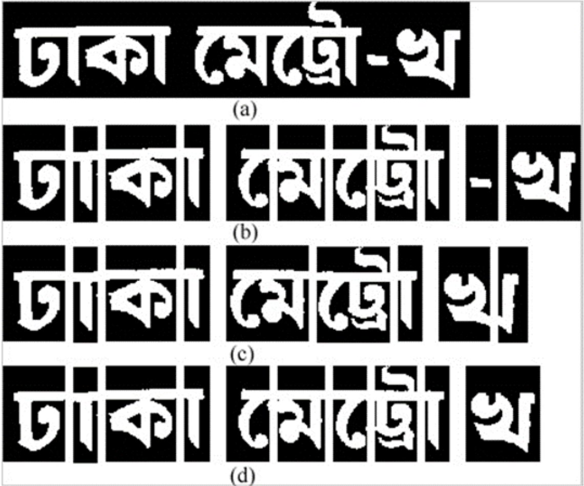
Figure 5.2: Character segmentation: (a) Original license plate, (b) Manual segmentation, (c) Segmentation with constant threshold 4, and (d) Segmentation with adaptive threshold (Algorithm SAT).
