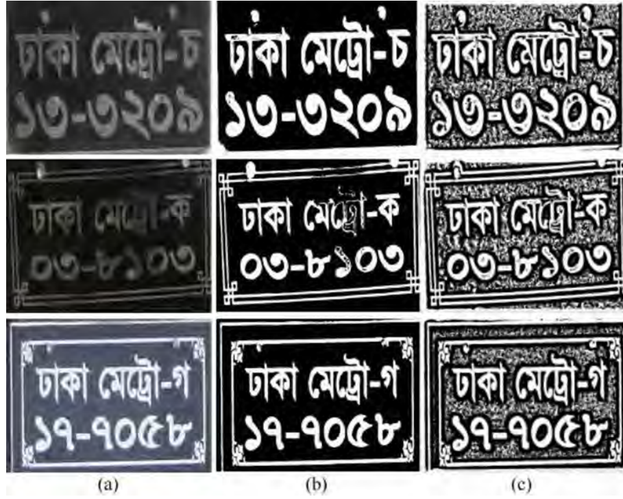
Figure 2.3: (a) Original input images, (b) Binarization using Otsu's algorithm, and (c) Binarization using Sauvola Algorithm.
