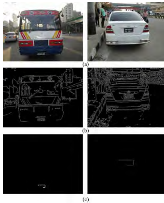
Figure 5.1: License plate detection: (a) Original input images, (b) Edge images, and (c) After the application of symmetry detection algorithm and ROID.
