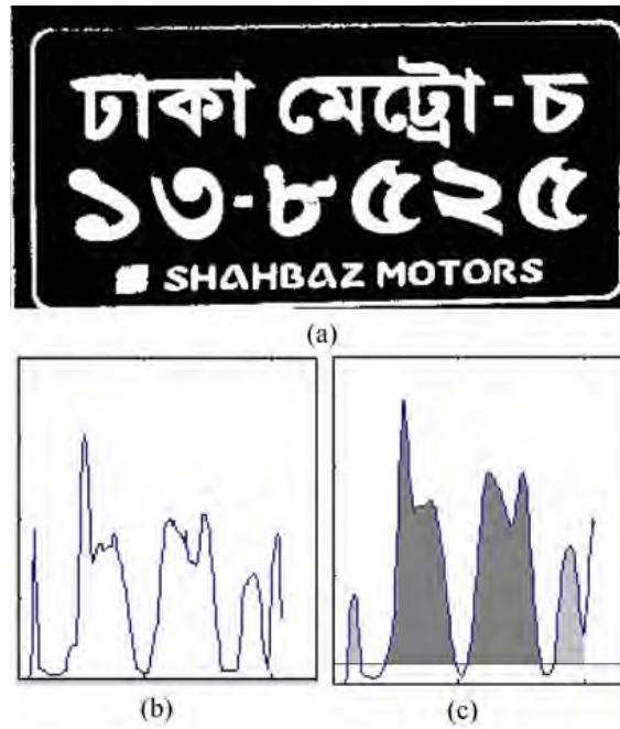
Figure 4.13: Outputs of simple license plate License segmentation stage. (a) Binary image of a simple license plate, (b) Horizontal projection of the pixels, and (c) Filtered projection.
