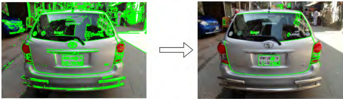
Figure 4.6: Sorting contours keeping minimum area as 30 pixels
