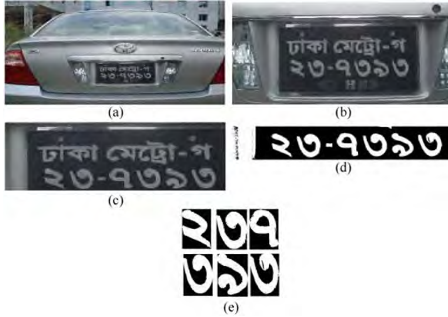
Figure 3.6: (a) First picture, (b) Empirical crop result, (c) Brute force and scanning result, (d) Registration plate with only the lower half, and (e) Extraction of individual characters.
