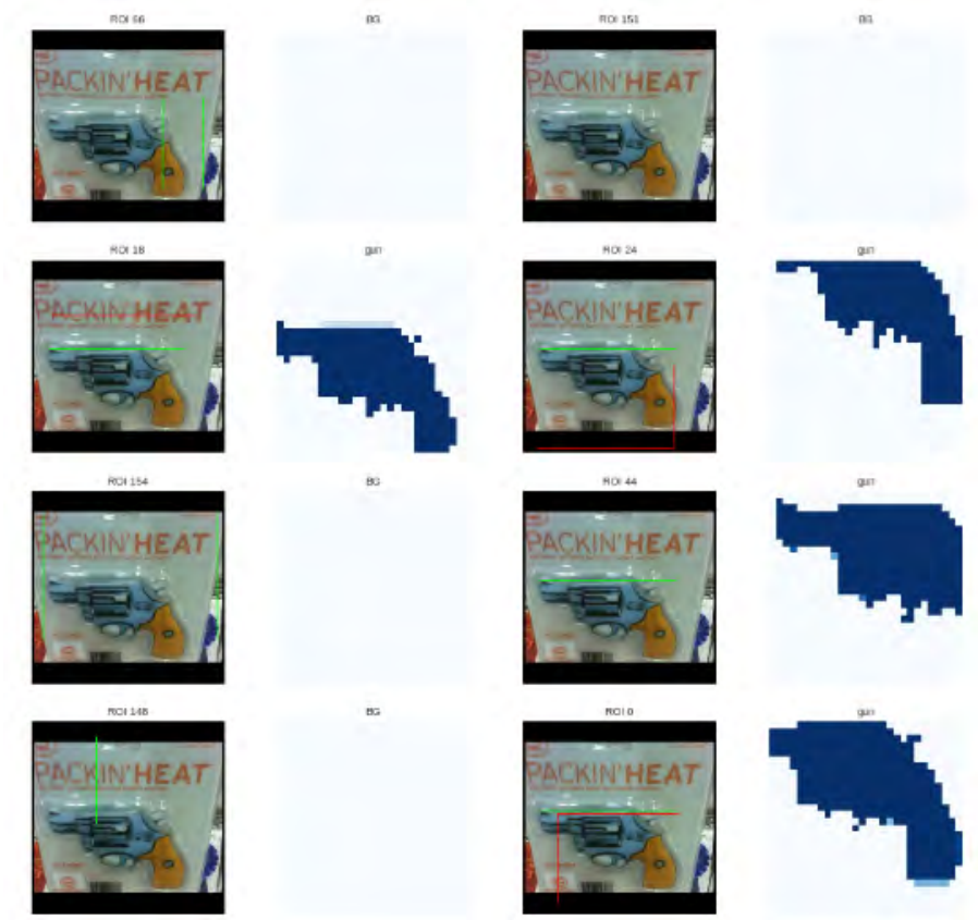
Figure 5.5: Positive and negative ROI analysis with positive to negative ROI ratio during training. The figure also shows that the network can create unique ROIs and that this is due to the lack of redundancy and to the efficacy with which the network covers a range of such object regions.
