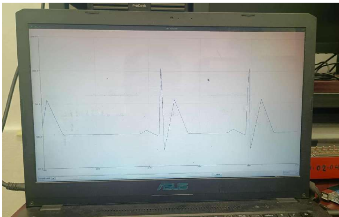
Figure 5.69.6: ECG signals as corrected by the single pacing signal on the far left
