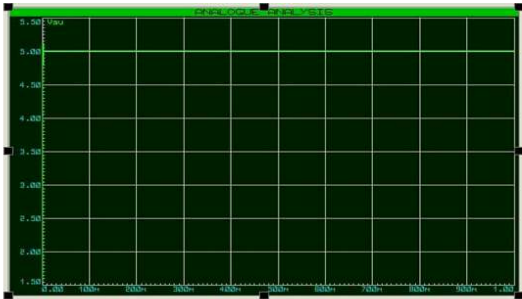
Figure 4(1j): 5V DC output of the Supply Unit for other modules.
