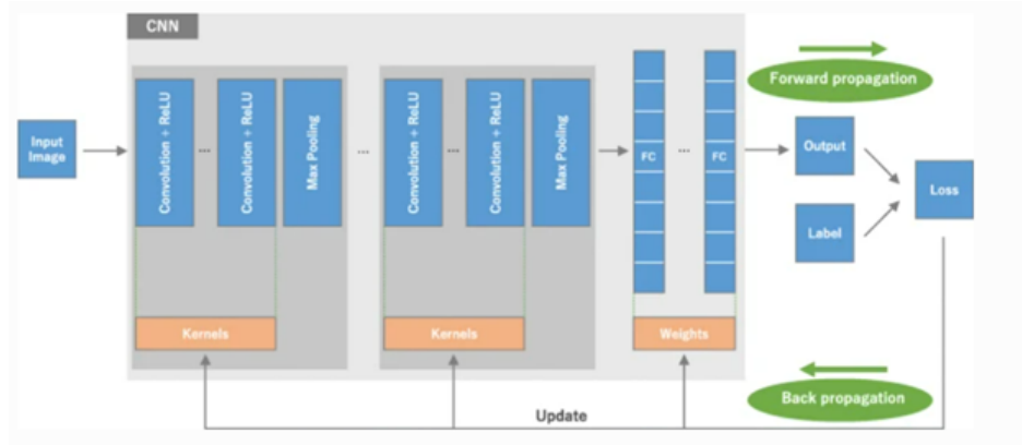
Figure 4.1: Convolutional neural network (CNN) architecture and the training processes with forward and backward Propagation layers
