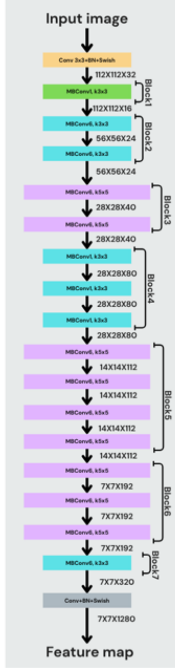
Figure 4.4: Architecture of EfficientNet-B0
