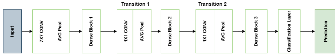
Figure 3.7: DenseNet121 model architecture.
