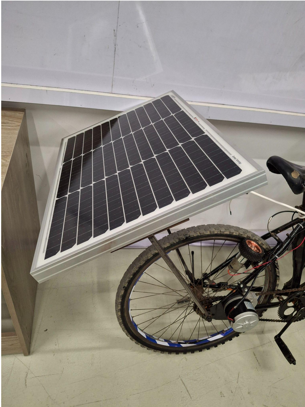
Figure 5.8 : Hardware Solar panel Installation
