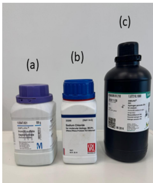
Figure 2.3 : Reagents used in the experiment. a) Iron sulphate heptahydrate, b) Sodium Chloride c) Hydrogen Peroxide
