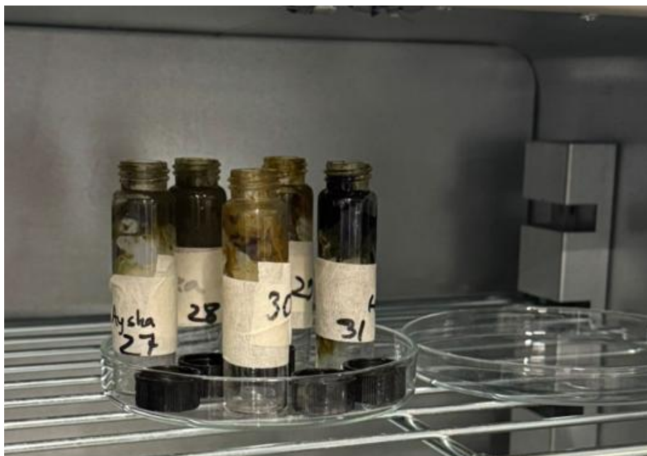
Figure 2.10 : Samples were placed in a drier at a constant temperature of 40°C to remove all moisture .
