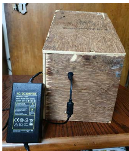
Figure 26: Supplying Power with AC/DC Converter to Home Unit
