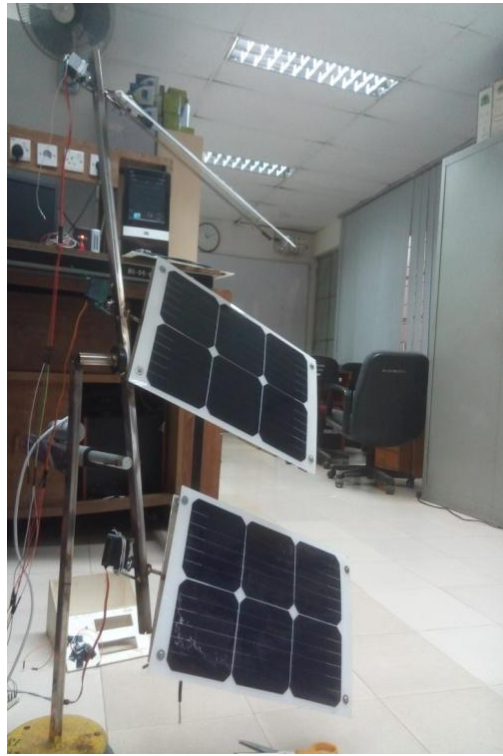
Figure 2.5: The way servo motors are attached with the solar panels in the system.
