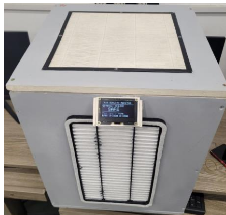
Figure 66: CCU Showing “Safe”; Fan OFF
