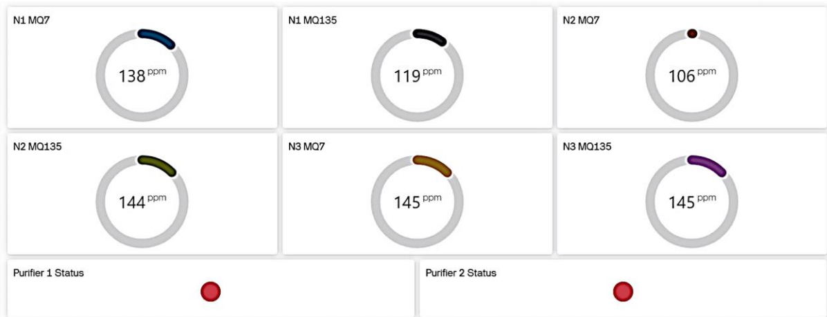
Figure 21: Purifiers are ON at High and Medium Pollution Levels (Blynk Interface)
