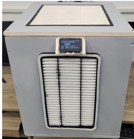
Figure 63: CCU Showing “Low”; Fan at 80% Speed
