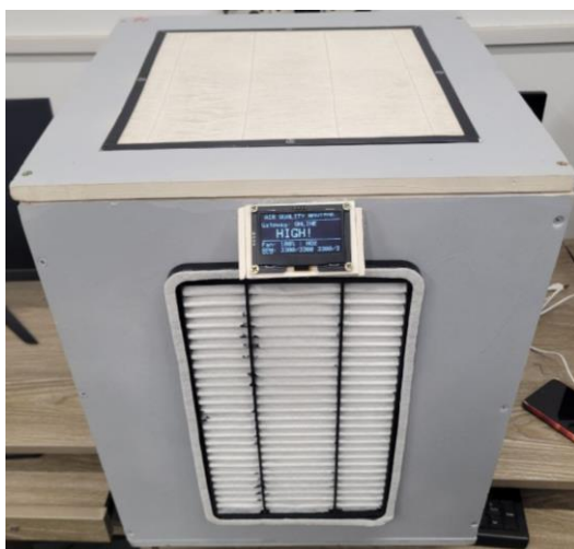
Figure 57: CCU Showing “High”; Fan at 100% Speed
