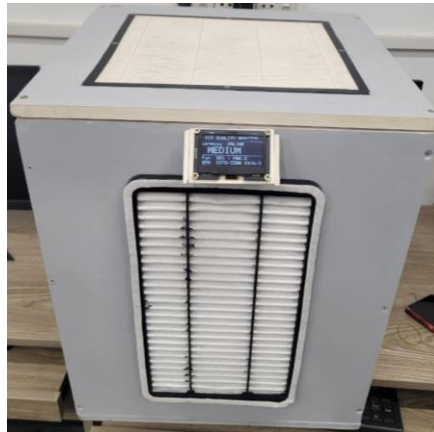
Figure 60: CCU Showing “Medium”; Fan at 90% Speed
