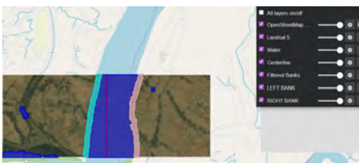
Figure 4.11: Could detect left/right bank accurately when there is no char
