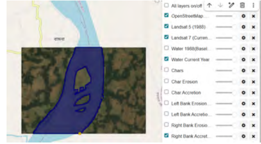
Figure 4.27: Right bank Accretion with Respect to the Base-Year (1988) Water Body
