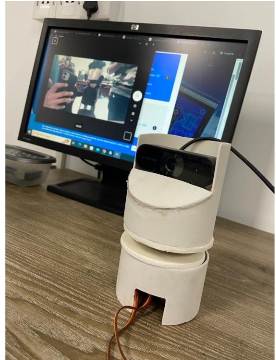
Figure 23: Integration of servo and camera mechanism with outer shell.
