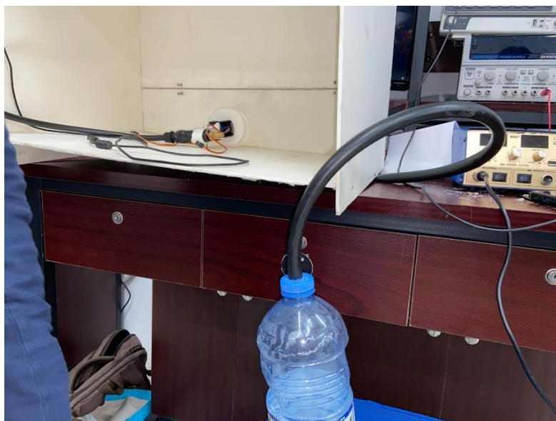
Figure 26: Water drainage system and tank
