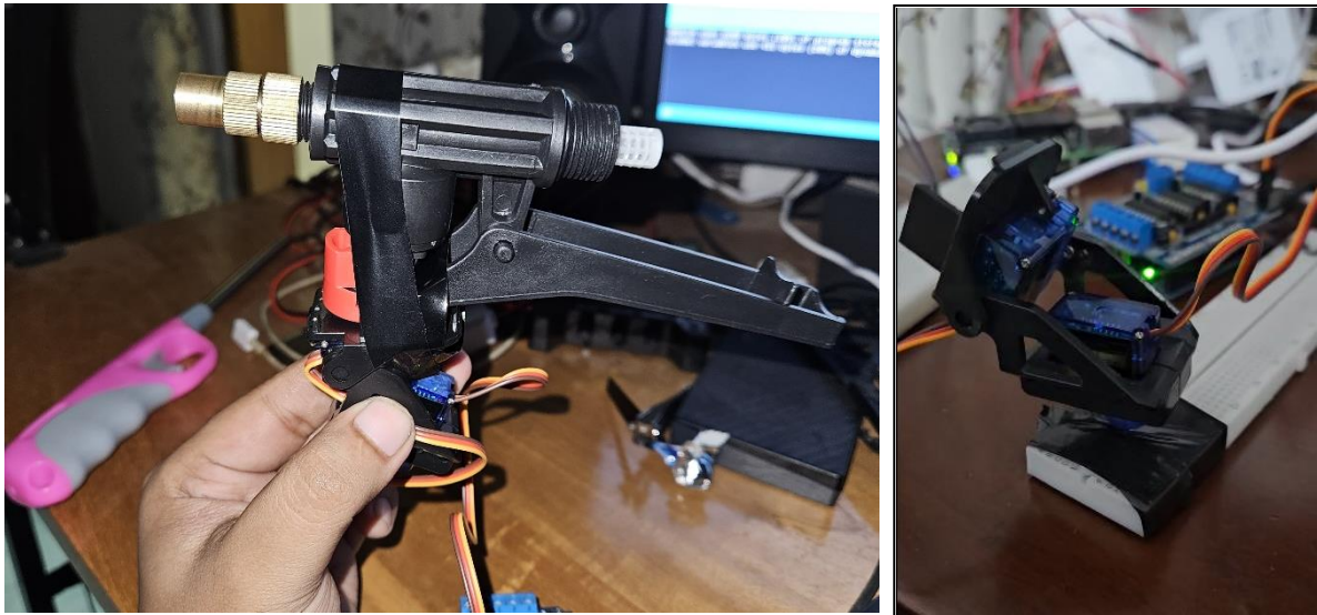
Figure 21: Water Nozzle and servo motor
