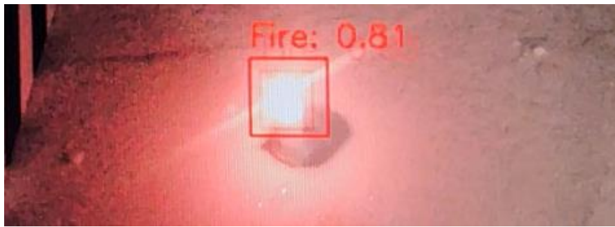
Figure 34: Fire hazard detected by the CNN model.
