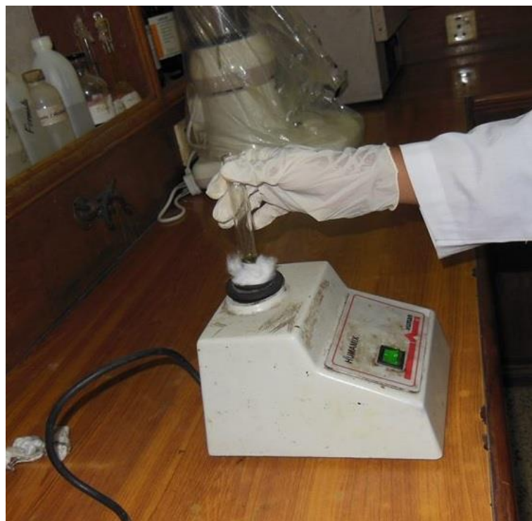
Fig. 3.4. Preparation of the solution of plant extract with the help of vortex apparatus.
