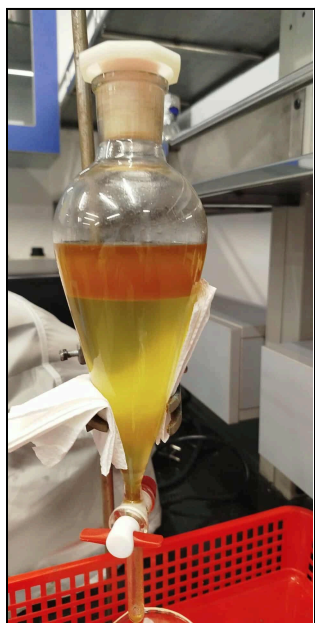
Figure 3.1.4.1: Chloroform solvent-solvent partitioning of Moringa oleifera leaf (upper part: organic phase, lower part: aqueous phase)
