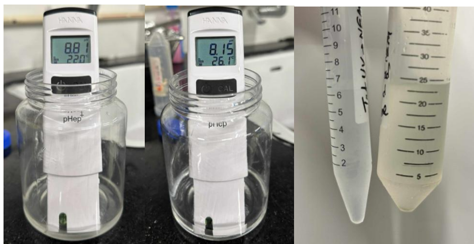
Fig 3.16: After the treatment, treated sample pH 8.15 & untreated sample pH 8.81, significant color change in the water is visible.
