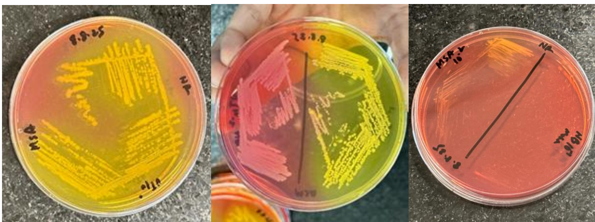
Fig 3.8: Untreated water sample showed various yellow and red colonies, whereas treated sample contains no growth of bacteria in the MSA agar
