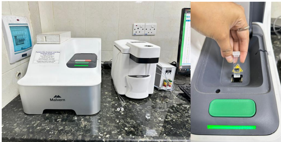
Fig 2.2: Malvern Particle Analyzer for Nano bubble size measurement
