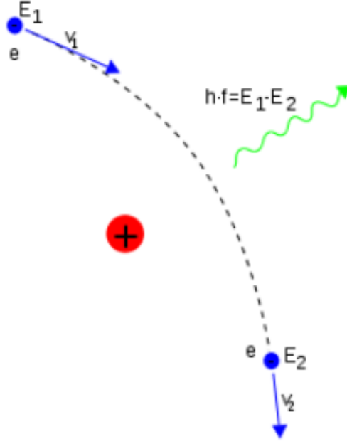
Figure 3.1: Bremsstrahlung radiation is depicted in a simple schematic design. While passing near a proton, an electron (blue) slows down (red). Because it loses some energy ( E_1 - E_2 ) via bremsstrahlung radiation, its energy ( E_1 ) and velocity ( v_1 ) before the interaction are greater than the energy ( E_2 ) and velocity ( v_2 ) after the encounter[36]
