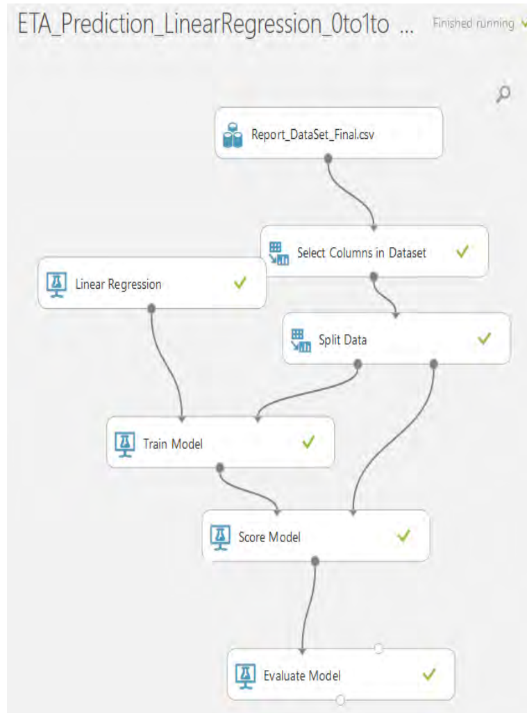
Figure 3.2.2 c: Linear regression flow chart model used in cloud
