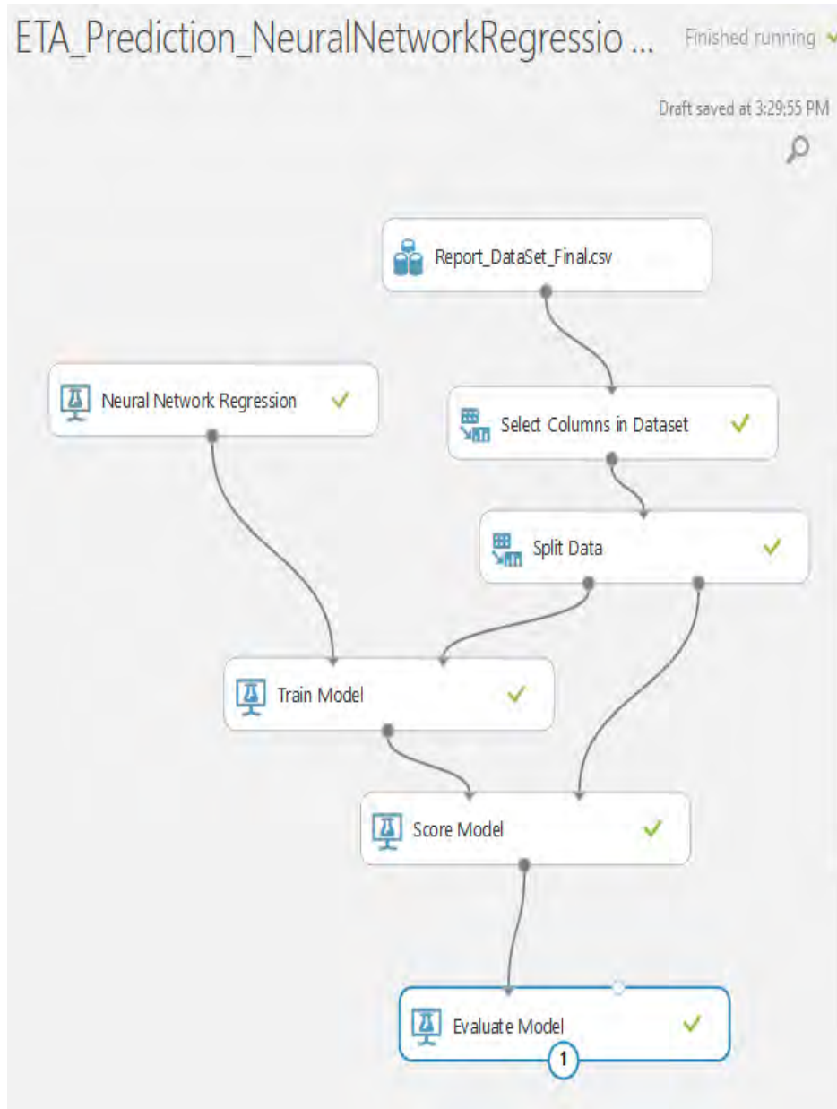
Figure 3.2.2 d: Neural network regression flow chart model used in cloud
