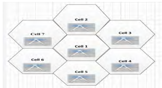
Figure 3.2: Cell in telecom network
