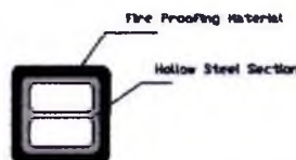
Typical Structural Member Section
