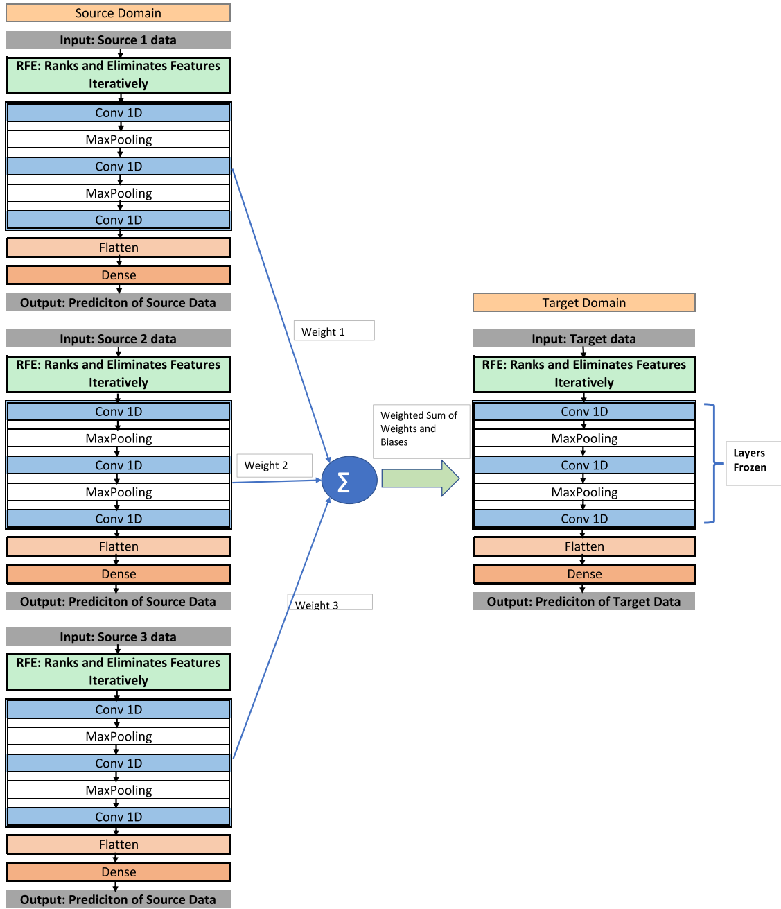
Fig. 8. Multi-source Multi-Layer TL network with RFE (MSML-TL-RFE).
