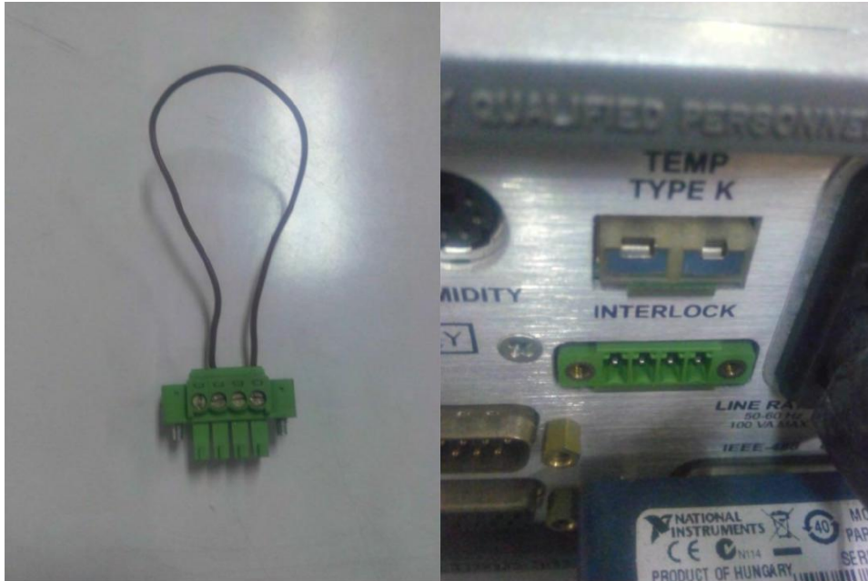
Fig 2.6: Interlock connector with pins 1 and 3 shorted (left) and the back panel showing interlock section (right)
