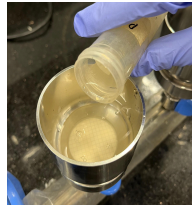
Figure 5: Each water sample was passed through the membrane filter
