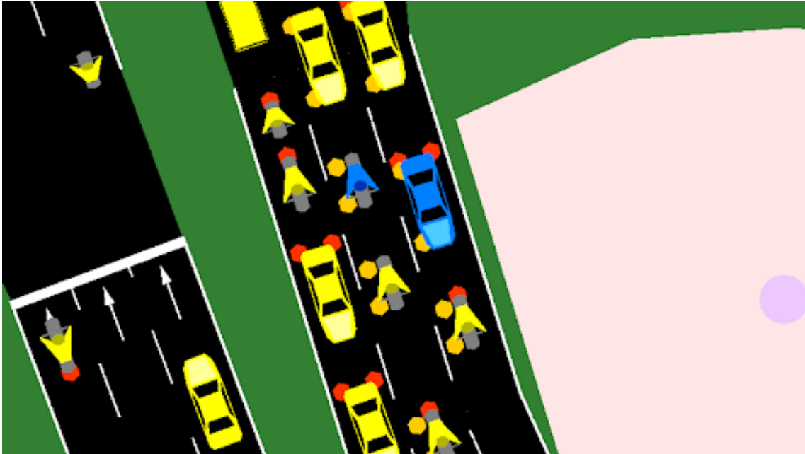
Figure 4.9: Simulation screenshot illustrating a jaywalking-induced slowdown. A vehicle on the main road is colored blue, indicating that a pedestrian crossing event temporarily slows it.
