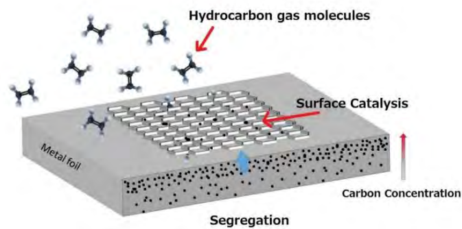
Figure 3.1 (b): Chemical Vapor Deposition - The high temperature causes the methane to break down into carbon atoms on the surface of the metal foil sheet. These carbon seeps underneath the surface and upon cooling, these carbon atoms resurface in layers and accumulate into a single sheet(s) [21][22].
