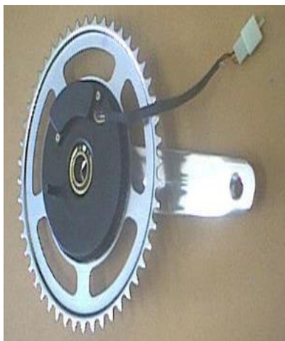
Fig 5.1 Torque Sensor with module
