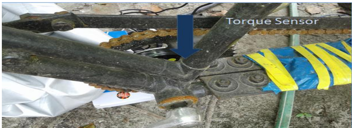
Fig: The torque sensor after being implemented
