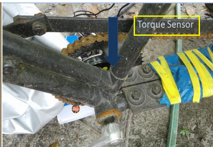
Fig 5.2 Torque sensor after being integrated
