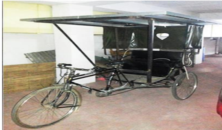
Fig 3.4: Electric Rickshaw with PV panel installed in ‘flat state’
